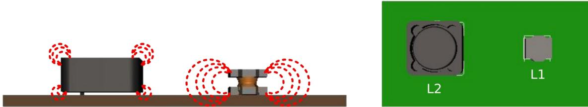
**Figure 2:** Magnetic field by shielded (L2) and not shielded (L1) inductors.
