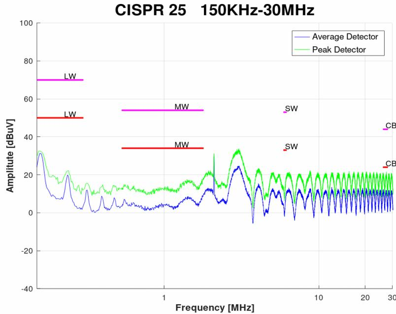
Figure 5: PCB coupling due to radiated field - board ID: 1-1 (BW: 150KHz - 30MHz).
