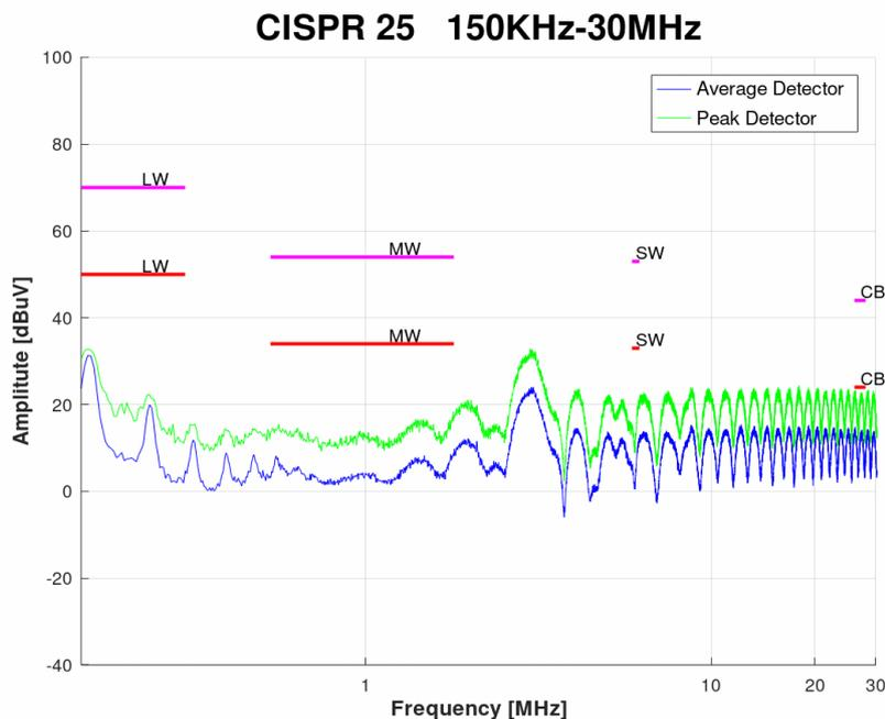
Figure 6: PCB coupling due to radiated field - board ID: 1-4 (BW: 150KHz - 30MHz).
