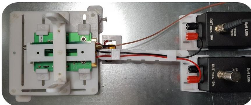
**Figure 4:** PCB test setup with ID: 1-1 on top of the DC-DC converter evaluation board.
