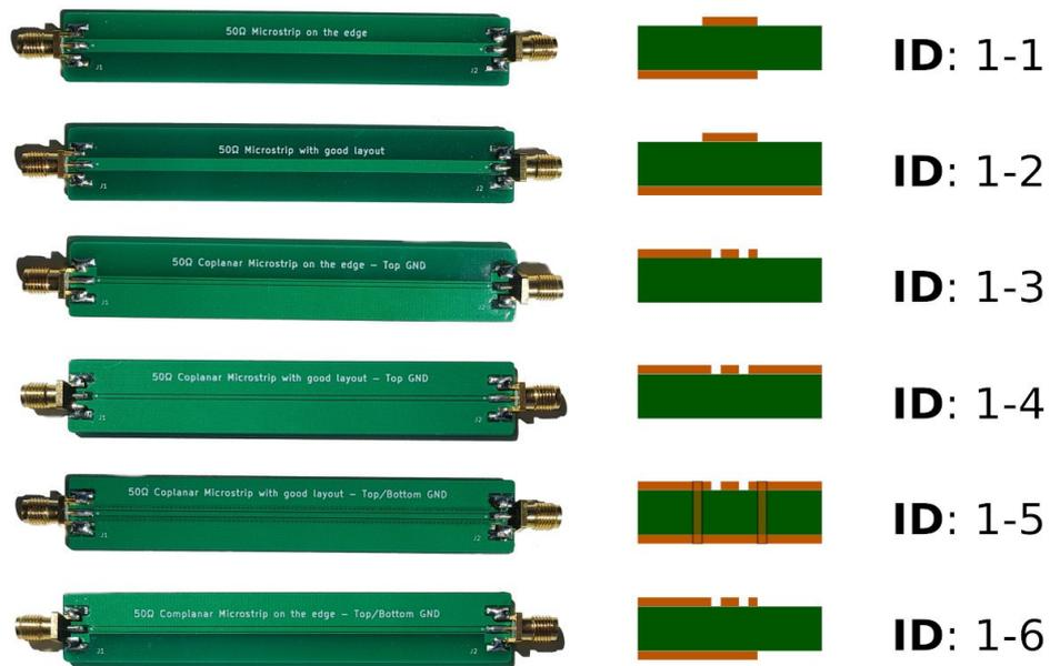
**Figure 1:** PCBs used for the tests. The transversal sections is shown for reference.
