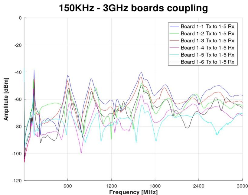
**Figure 3:** PCB coupling due to radiated field (BW: 150KHz - 3GHz).
