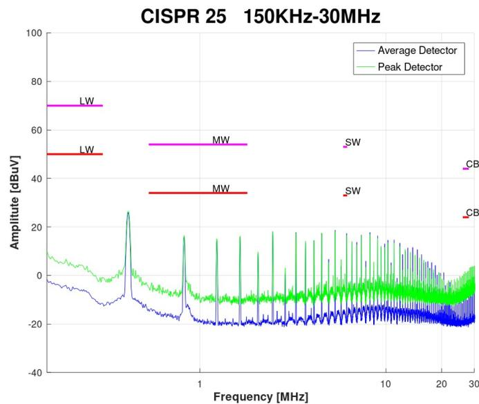
Figure 5: Conducted noise after applying an EMI filter.
