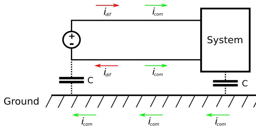
**Figure 1:** Conducted noise with the details of DM and CM contributions.
