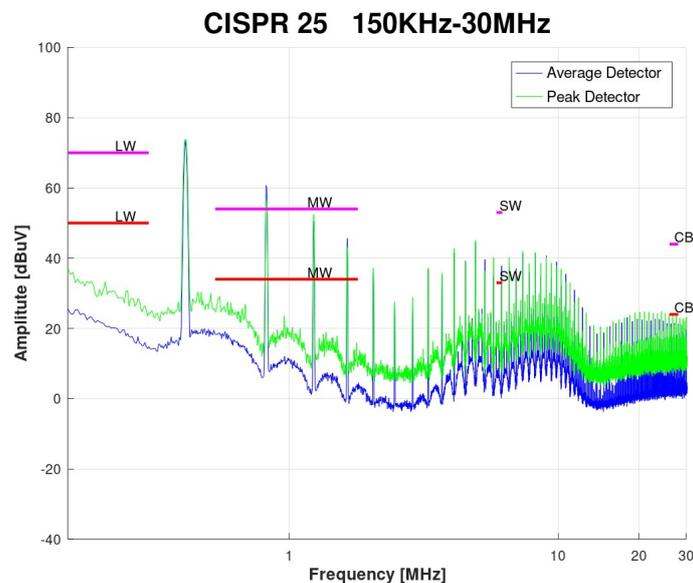
**Figure 2:** Total conducted noise for typical buck converter.
